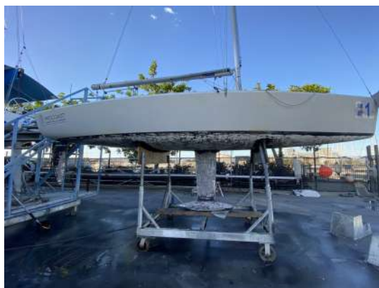
Above: F24, drying the bilges and removing any signs of mould. Waterproofing all deck fittings and penetrations, scraping off all of the old antifoul back to gelcoat and starting new.
