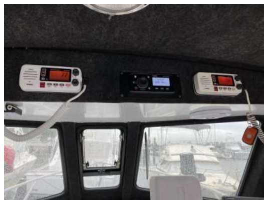
Above: The aluminium mark boat received a second VHF radio to monitor dual channels.
